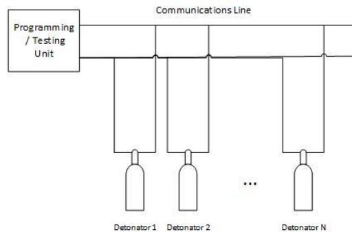
**Figure 3. Detonators connected to integrated programming/testing unit via a communications line**
