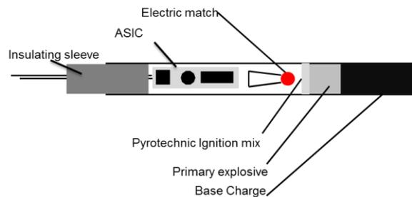
**Figure 1. Electronic delay detonator**
