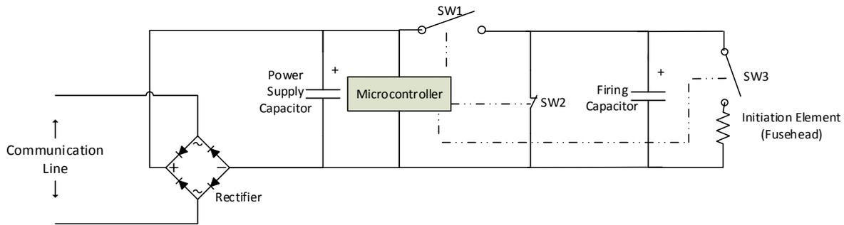
**Figure 2. Simplified electronic detonator circuit diagram**
