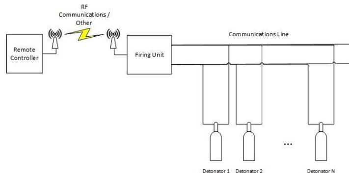
**Figure 5. Firing unit operated remotely via RF communications**
