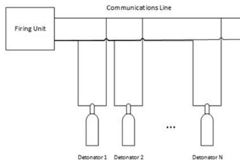
**Figure 4. Firing unit connected to detonators**
